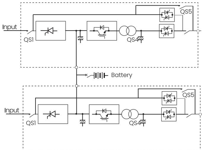
■ **Parallel UPS for Capacity or redundancy**
